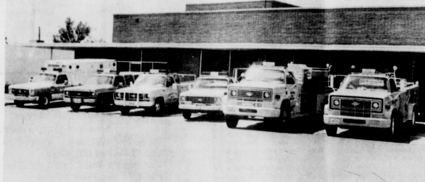
ABERNATHY EMERGENCY VEHICLES: Left to right, Ambulance; Chief's Car & Jaws of Life Vehicle; 1 ton booster pump; 1 ton booster pump; 750 GPM city pump and country pumper truck.
