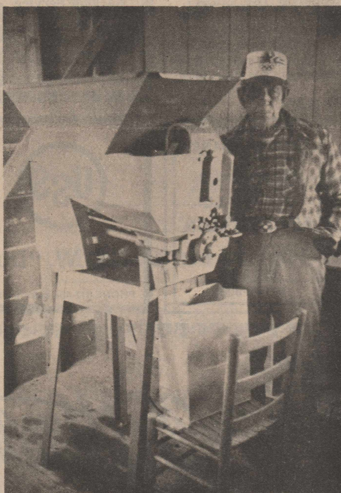
READY FOR pecans is Harry Hickman shown with his new Meyer Pecan Cracker and stand. Harry has one of the few commercial crackers in the immediate area and is keeping busy with this year's crop. The new machine loads from the hopper on top and each pecan is individually picked up and cracked, ready to pull the hulls apart and retrieve the pecan halves completely intact.
