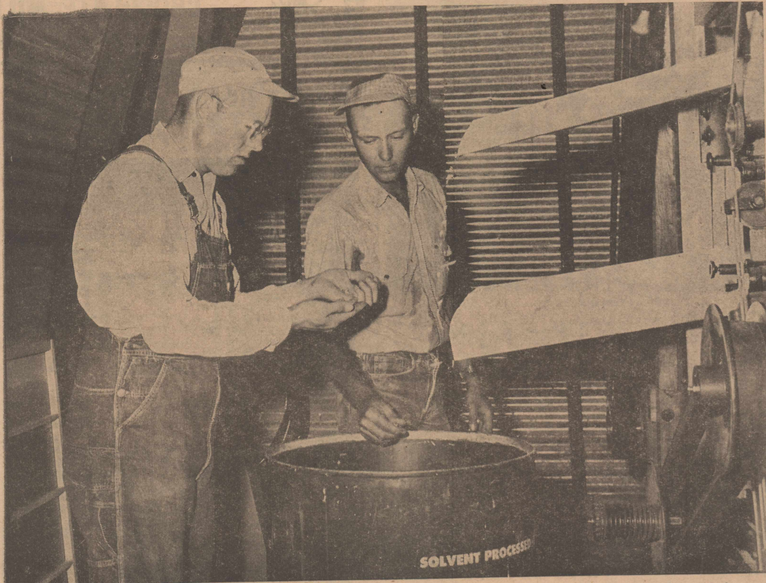
James Cowart, left, and Johnny Hodges keep a close watch on their Clipper Cleaner as it cleans their first load of the 1959 bean crop. The spout at the top sifts off cracked beans and the one below carries off trash. The beans being processed were produced by Buster Tanner. (STAFF PHOTO)
