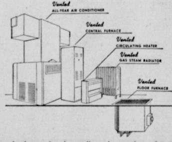
Proper heating requires that appliances be vented to a flue. The appliances illustrated above are types that are vented. For this reason your gas company recommends them, for only with heaters that are vented to a flue can you enjoy natural gas heat at its best. Only when appliances are vented are wall sweating and stuffy air eliminated. Plan healthful, modern heat-vented heat-for your new postwar home. Make sure there will be enough flues.
