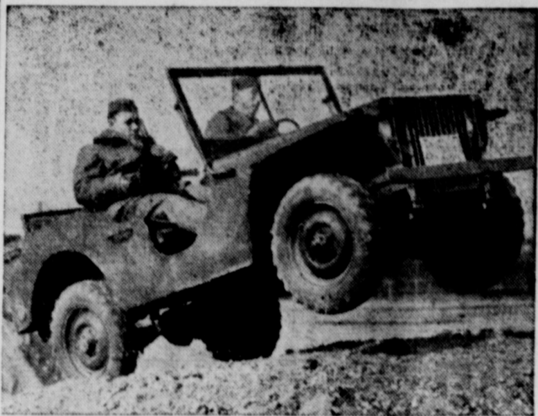
Speed shot at Camp Holabird, Maryland, during tests on new Light Reconnaissance and Command Cars for United States Army. They carry machine gun and crew of three men at approximately 60 miles an hour. Can climb steeper hills than tanks. The Ford Motor Company, which built the ditch-jumper shown above, has an army order for 1500 of these units.
