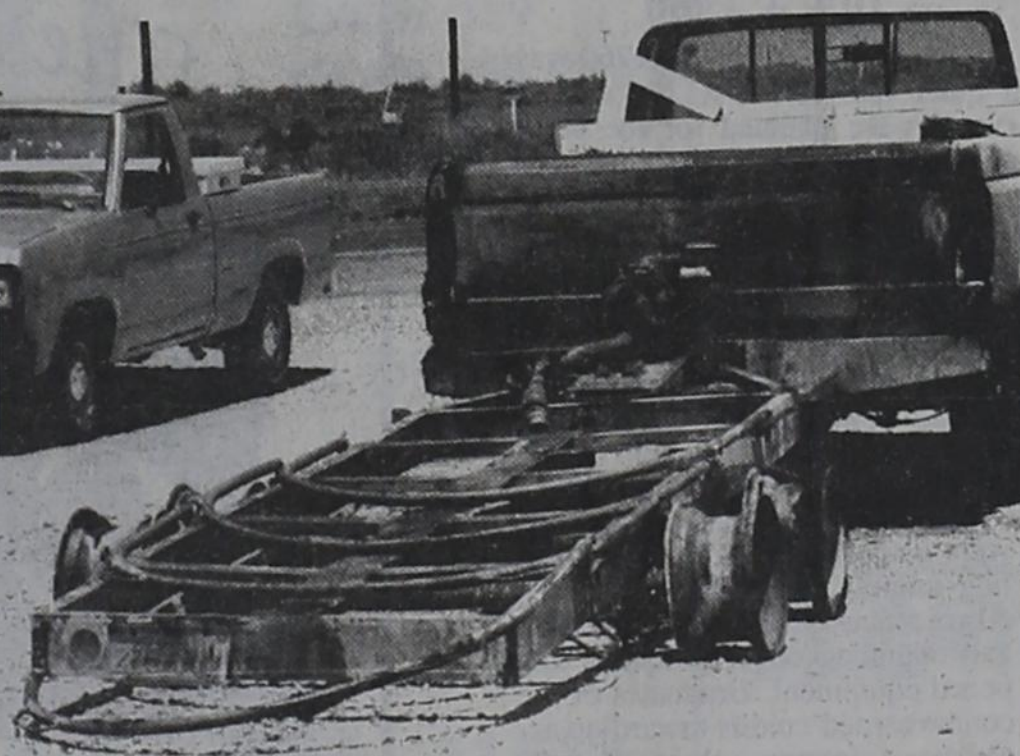
DEREK MILAM was treated and released at Methodist Hospital last week for second degree burns following the fire last Tuesday afternoon at Mid Plains gas processing plant on U.S. Hwy 84. According to witnesses, Milam was loading oil from a storage tank when the small gasoline powered engine powering a pump back-fired, igniting the fuel, which blew the trailer tank off its platform, melted the trailer tires, scorched the rear of the pickup truck and started a fire on the main oil storage tank.
