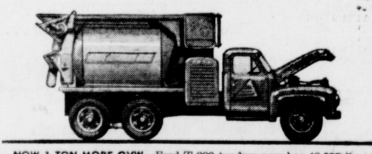
NOW 1 TON MORE GVW —Ford T-800 tandem now has 42,000 lbs. GVW. 170-h.p. Short Stroke V-8. 11,000-lb. front axle available. Increased capacities also apply to corresponding Cab Forward models.
