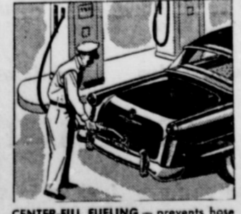
CENTER-FILL FUELING - prevents hose marks, and makes "filling up" easier from either side of the gasoline pump. Shorter gas filler pipe gives you trunk space for an extra suitcase.
