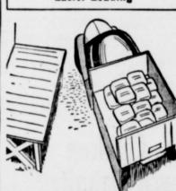
A farmer handy with tools can make a drop-side to his wagon or truck as illustrated above with a few pieces of scrap iron and a length of pipe. It will save considerable trouble loading and unloading, especially when the truck is pulled close to a loading platform.
