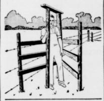
Here is the answer for a walk through gate for a barbed wire fence. Three extra posts, a few boards and two hours of your time are the essentials. The 2x4 nailed across the top takes the place of two braces. Located at convenient points on your farm this type of gate will save time and prevent that business of getting down on the ground and rolling under barbed wire.
