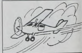
Most light planes are capable of taking off or landing in 90-degree crosswinds that are less than 20 percent of the airplane's power-off stall speed.
