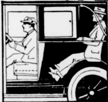
Front seat adjusts to three positions to accommodate short driver or tall driver.
