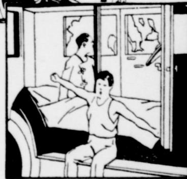
Both seats and upholstery make into a full-length, full-width bed in car for camping.
