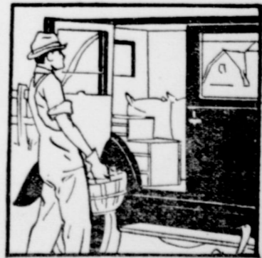
50 cu. ft. of space for farm produce, luggage, etc., by removing rear seat and upholstery.
