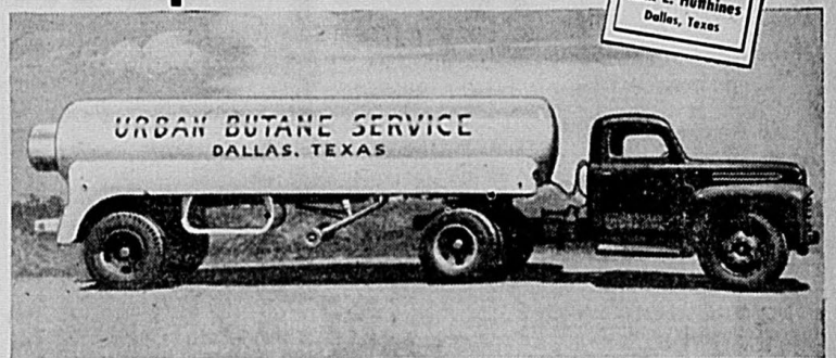
Ford Model F-7 BIG JOB shown has Gross Combination Weight rating of 35,000 lbs. as a tractor; Gross Vehicle Weight rating of 19,000 lbs.
