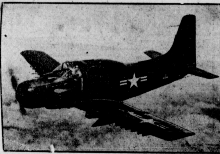
MULTIPLE USE BOMBER —Built by Douglas for the U. S. Navy, this is the new AD-5 Skyraider "Multiplex" bomber, said to be the most versatile airplane ever to fly. Embodying a new design concept, basic Skyraiders are produced as a "universal chassis," along with packaged conversion kits. Aboard Navy carriers, they may be converted to any one of a dozen different combat types according to immediate need. This "13-in-1" utility aircraft supplies the fleet directly with a 'basic attack plane; photographic plane; tow-target plane; passenger plane; ambulance transport plane, and a variety of radar planes.
