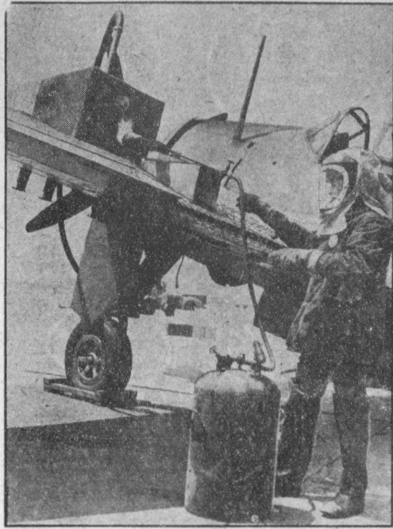
TRIAL BY FIRE—A newly-developed gas tank for aircraft gets a blowtorch test by an aviation mechanic at Floyd Bennett Field in New York. Capable of withstanding direct flame and intense heat up to 2000 degrees Fahrenheit, the specially coated tank failed to burn after being exposed to the blowtorch flame for 28 minutes. A conventional gas tank bursts into flames after less than two minutes.
