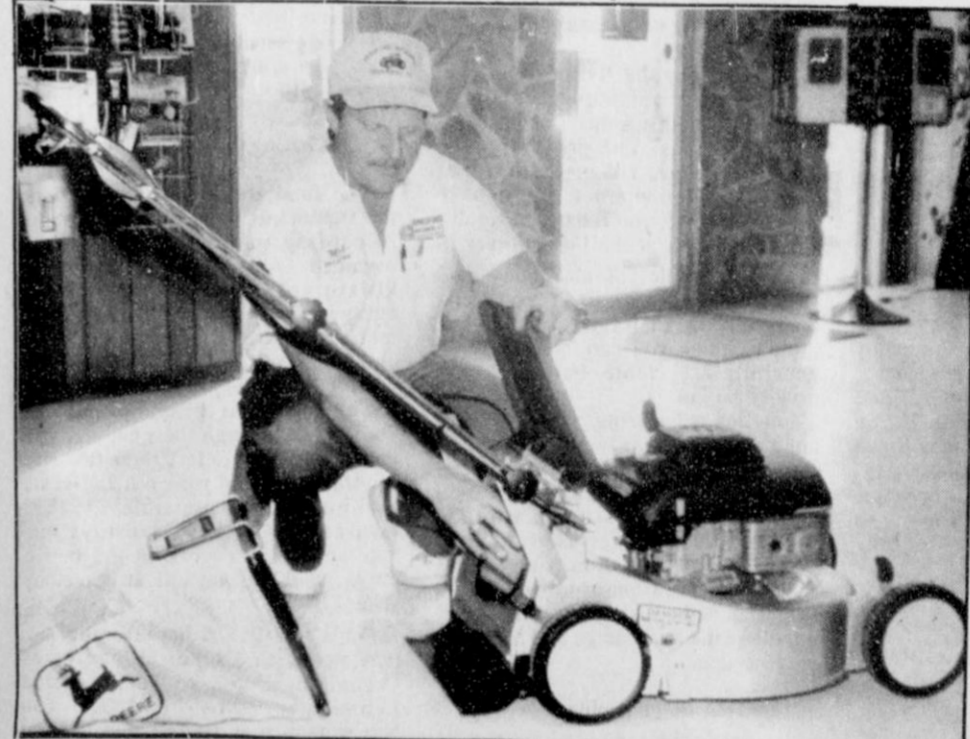
Mark Schoenhals of Hansford Implement demonstrates how placing a plug at the back of this mower will force grass clippings into the blades. This will produce a mulch.
