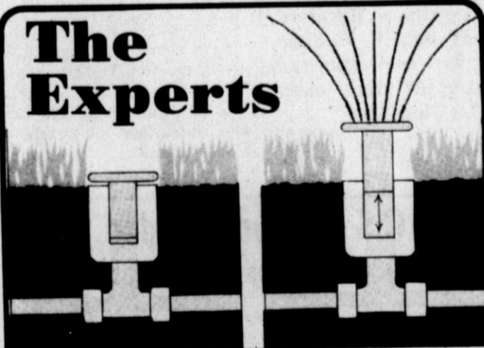
UNDERGROUND SPRINKLER SYSTEM
