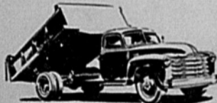
HEAVY-DUTY CAB-AND-CHASSIS with Dump Body Model 6403—161-inch Wheelbase Maximum G.V.W. 16,000 lb.
