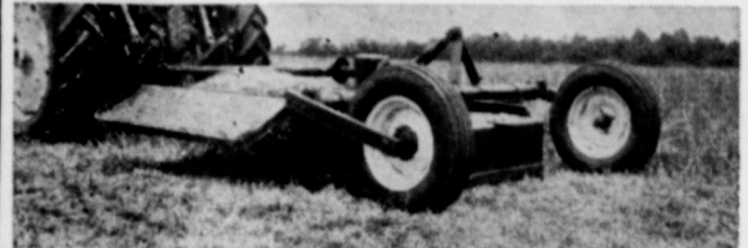
Makes hay as fast as your tractor will go. Side member adjusts to 45 degree angle (as above) or 90 degree angle to spread heavier material for drying.
