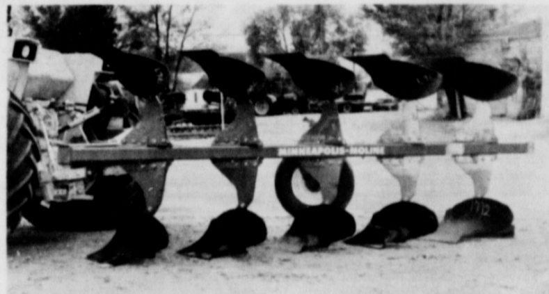
MINNEAPOLIS-MOLINE 5 BOTTOM PLOW 14 To 18 Inch Cuter Bottom From 3 to 5 Bottoms Spinner Type Semi Mount On Mounted
