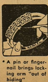
A pin or fingernail brings locking arm "out of hiding"
